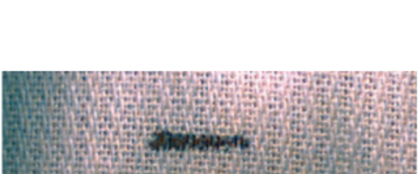
Faultless beams coming out of a good weaving preparation room, experienced and trainable staff, use of quality materials, periodical maintenance will be helpful in coping with stop marks.
